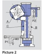
Pressure in P2 (indexing) The locator B retracts and releases the indexing shaft A; the finger C moves forward and rotates the shaft by 45°.
