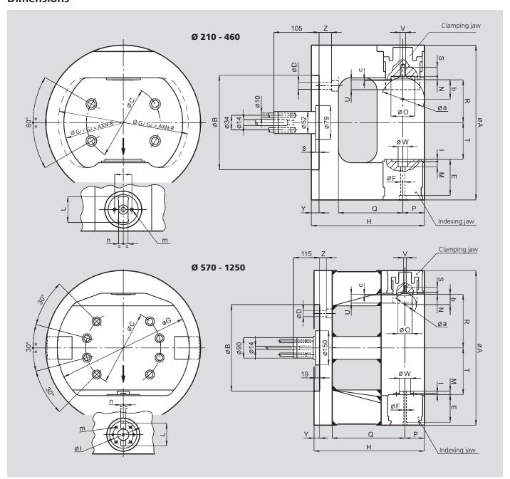
AXN-R Automatic indexing chucks, reinforced Ø 210 - 315 mm
