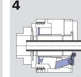
Centering jaws open and retract back axially into the chuck body. The pipe can now be machined.
