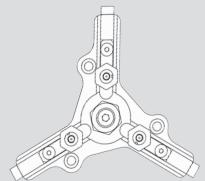
Determination of height of locator posts:  $\Delta$  = Distance between clamping position and locating face Height of locator posts [H] = 32,5 mm -  $\Delta$
