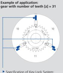
Specification of Key Lock System: 1x Key straight, 2x Key for number of teeth 31
