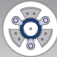
Swing-clamps swivel inward + clamp axially. Centering jaws open (if requested)
