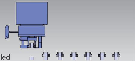
**Radial clamping only is also possible = function like D-chuck**
