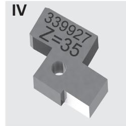
One set of Key Lock insert consists of 2 keys. Gears, which number of teeth that is divisible by 3 can be machined with 3 of the same type Key Lock insert (straight). For all gears, which number of teeth is not divisible by 3, there are different key insert sets available according to the number of teeth. The Key Lock inserts are the same for all 6 sizes of top jaws.
