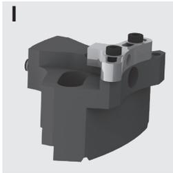
At first you need to choose your matching top jaw (size 1 - 6) for the outside diameter [ $d_a$ ] of the gear to be machined. Each size of top jaw can cover 20 mm outside diameter using two different types of clamping pins (Type A and B). One set of top jaw consists of 3 pieces including 1 straight key lock insert.
