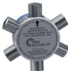
Separate measuring head for 2, 3 and 6 jaws
