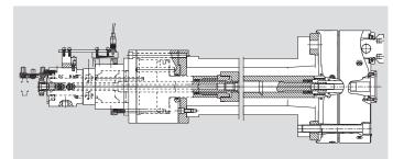
■ TSX-C: chuck operated with a DCE cylinder with central bore for air sensing or coolant flush (only 1 media).
