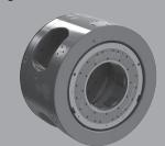
Hydraulic ring indexing chuck for threading of couplings in **1 set up** with the original SMW Type SF-RAZ (6 jaw clamping: 3 jaw self centering, 3 jaw compensating).
